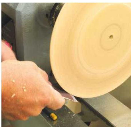
▲ Pic.16 Remount the blank on the chuck after truing up the face texture of the top for about a third of the diameter. This can cause the edge to get sharp in places so round it off with a piece of 80 grit
